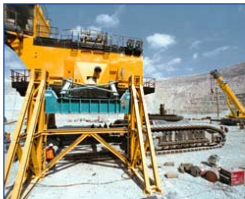
BACHMANN TURNER OVERDRIVE: Martin Bachmann Keller's computer-controlled hydraulic hoists takes a chunk out of shovel maintenance time
